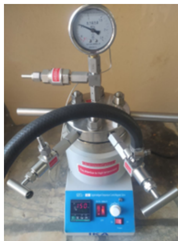
Figure 1 Photo of the container – high-temperature reactor
