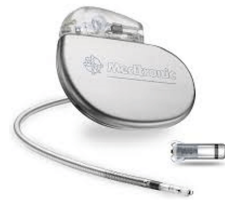
Figure 1 Diagram of a single-chamber pacemaker [8]
