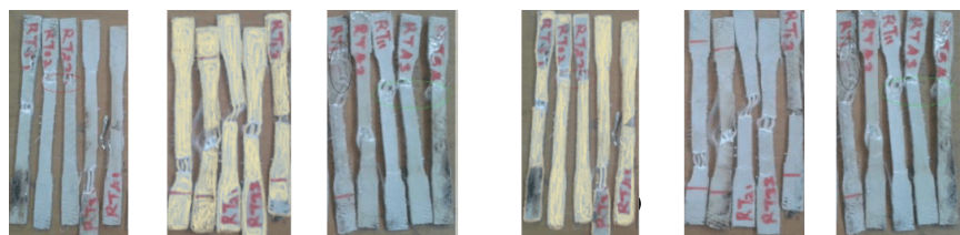
Figure 16 Tensile test results for different stacking sequence (a) Glass-Sisal-Glass, (b) Sisal-Glass-Glass.
