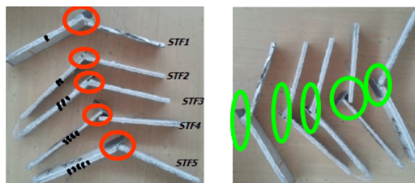
Figure 17 Failure modes after shear testing of results ABSSSJ specimens adhesive debonding
